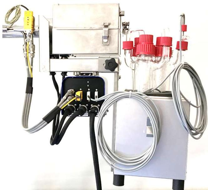
*Probe module on sampling probe*
