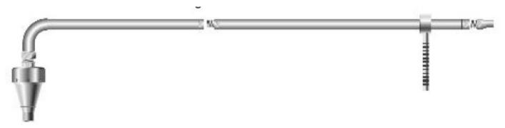
The curve of 90° allows assembling the filterholder in parallel in the gas flow, that enables simple sampling and reduced rinsed volume, which reduces incertainty for low concentration measurement.
